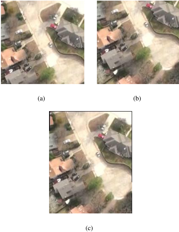
Figure 5: (a) First camera image, (b) Second Camera, (c) Final Mosaic (Affine Transformation)
